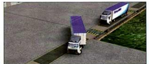
Résor@il loading schematic. (Note: tractor heads would drive off after positioning the trailer)
